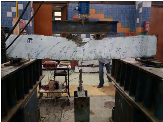
Fig. 4. Crack propagation of beam B1.
